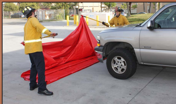
Working together, trap air under the cover by moving forward and backwards once or twice
