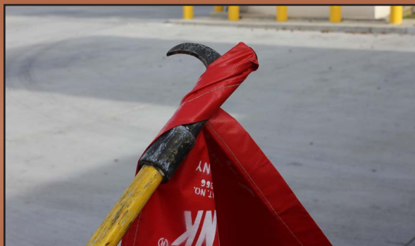
Place two pike poles through the corner grommets and twist around once, be sure to not puncture the cover with the hook
