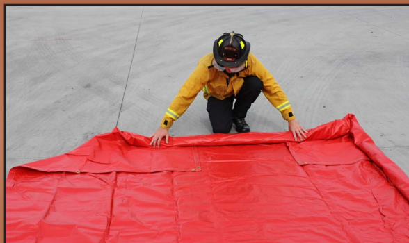
Repeat the previous step on all sides of the catch-all, rolling the sides inward approximately 2' to 3'
