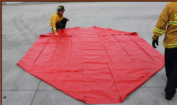
Spread out cover using two firefighters. Fold each corner inward approximately 3' to 4'
