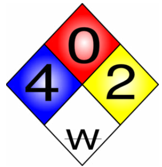
Figure 23-4 NFPA 704 Placard will indicate if material is water reactive
